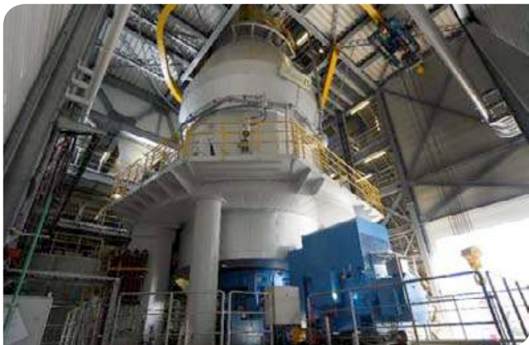
Above - Figure 2: The Loesche type LM 46.2+2 S VRM at the EQIOM Ciments plant in Dunkerque, France. See Case-study 1, overleaf.
