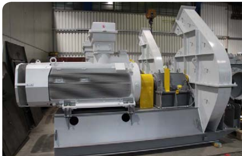
Below - Figure 4: A typical high-pressure fan made by Germany's Pollrich.
