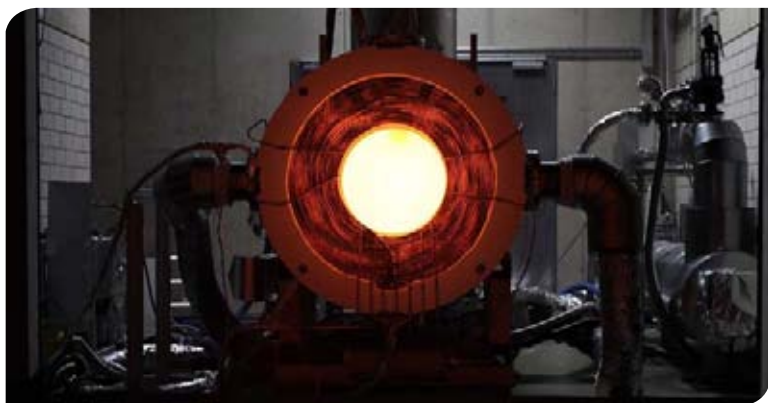
Above: A 250kW solar receiver developed by Synhelion has recently achieved gas temperatures in excess of 1550°C, opening up the prospect of cement production with an 'invisible flame.'
