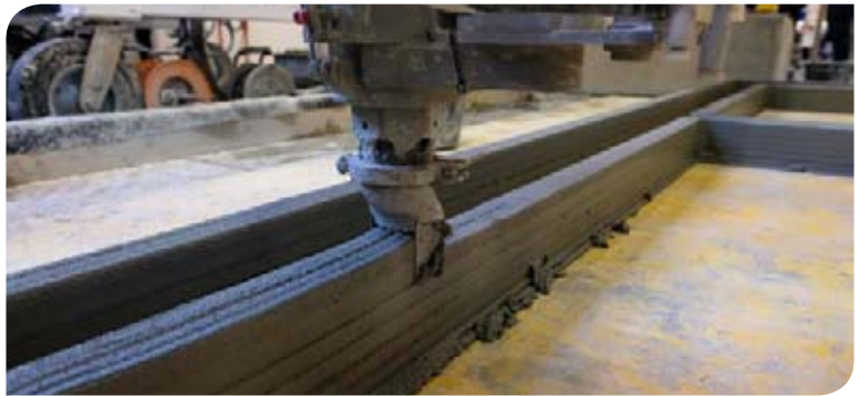
Above: The BOD 2 Printer can print smooth surfaces rapidly.
