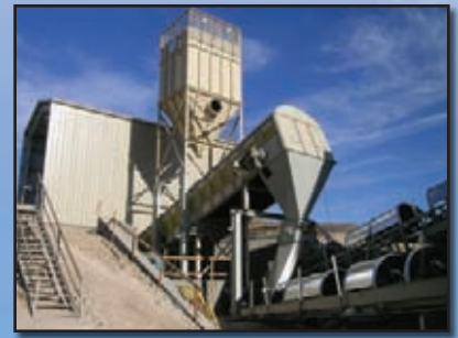
Truck Unloading Stations Receiving up to 1,200 t/h
